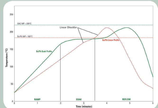
The stated profile applies to Sn63 and Sn62 alloys. This can be used as a general guideline in establishing a reflow profile when using **NC-SMQ® 92J Solder Paste**. Deviations from these recommendations are acceptable, and may be necessary, based on specific process requirements, including board size, thickness, and density. Start with the linear profile, then move to the optional soak profile, if needed. The flat soak portion of the linear profile (linear shoulder) may also be eliminated.
