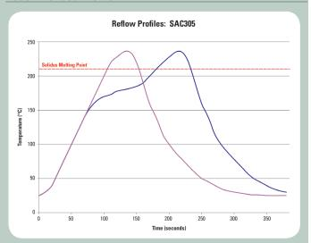
A short preheat ( $150-160^{\circ}$ C) for less than 45 seconds may be used to reduce voiding. The profile should ideally be a linear ramp at  $1-2^{\circ}$ C/second up to  $20-30^{\circ}$ C above solidus temperature, with a rapid cool down afterwards, and a minimum time above liquidus of 20 seconds.
